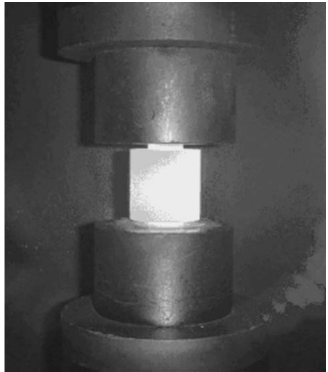
Fig. 2 Spark plasma sintering in operation as demonstrated by the glowing graphite die and punch set. The plasma sprayed sample is packed within the die using ceramic powders.
